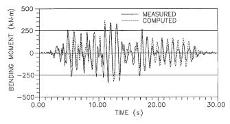
**Fig. 9.** Comparison between measured and computed bending moments at peak pile deflection for the single pile.
