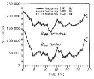
**Fig. 19.** Variation with time of (a) stiffnesses  $k_{vv}$  and  $k_{v\theta}$  of the four-pile group at f = 1.91 Hz, and (b) peak displacements at the pile cap.
