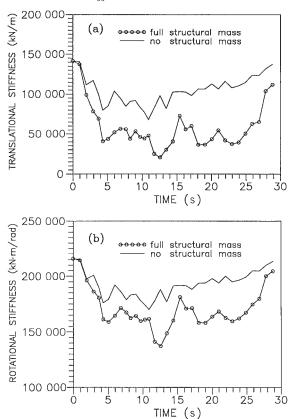
moduli and damping ratios of soil were obtained. Dynamic impedances of the pile foundation were computed again using the new sets of soil properties. The effect of the structural mass on dynamic stiffnesses of the pile foundation can be seen by comparing the translational and rotational stiffnesses of the pile foundation with and without the structural mass shown in Figs. 20a and 20b.
