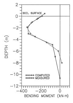
moment predicted by the quasi-3D finite element analysis is 344 kN·m, compared with a measured peak value of 325 kN·m.
