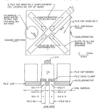
gravity of  $I_{\rm cg} = 715.39 \, {\rm Mg \cdot m^2}$ . The centre of mass of the total pile cap assembly is 0.96 m above the top of the pile cap, and the free-standing pile length is 1.21 m (Gohl 1991).
