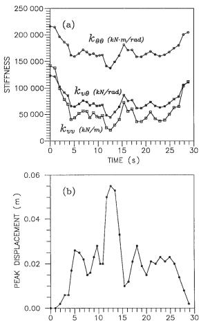
The variations of translational stiffness  $k_{\rm vv}$  and rotational stiffness  $k_{\theta\theta}$  with time at different excitation frequencies are shown in Fig. 18. It can be seen that the excitation frequency has little influence on the dynamic stiffness of the pile foundation for frequencies less than 10 Hz. Therefore, the dynamic stiffnesses of the pile foundation may be considered independent of frequency under seismic loading.
