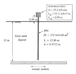
Fig. 5. The finite element modelling of the single pile.
