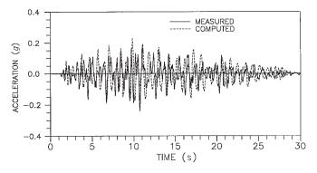
pile cap is 0.23g, which agrees very well with the measured peak acceleration of 0.24g.
