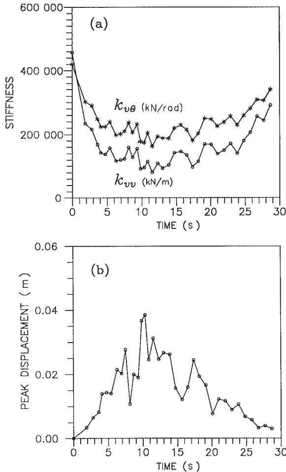
conducted to explore the effect of structural mass on dynamic stiffnesses of pile foundations. The centrifuge tests of the single pile presented earlier were reanalyzed without taking the structural mass into account. A set of time-dependent shear
