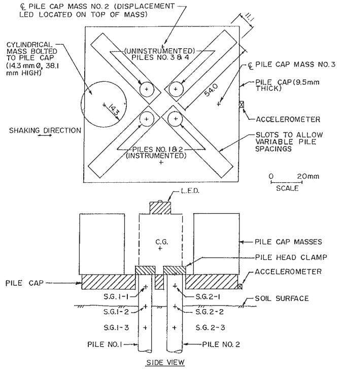
gravity of  $I_{cg} = 715.39 \text{ Mg}\cdot\text{m}^2$ . The centre of mass of the total pile cap assembly is 0.96 m above the top of the pile cap, and the free-standing pile length is 1.21 m (Gohl 1991).
