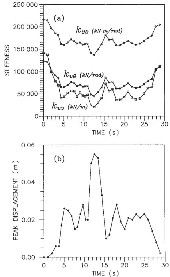
The variations of translational stiffness  $k_{vv}$  and rotational stiffness  $k_{\theta\theta}$  with time at different excitation frequencies are shown in Fig. 18. It can be seen that the excitation frequency has little influence on the dynamic stiffness of the pile foundation for frequencies less than 10 Hz. Therefore, the dynamic stiffnesses of the pile foundation may be considered independent of frequency under seismic loading.
