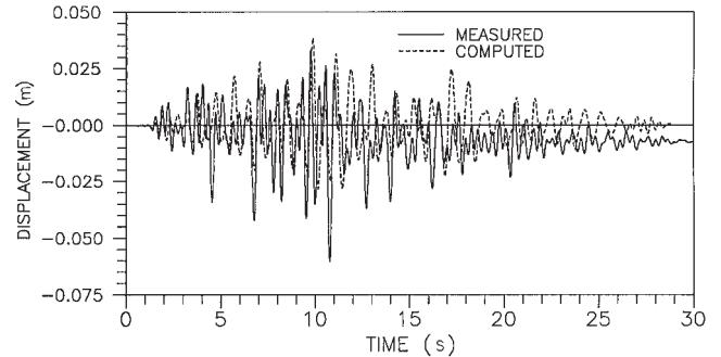
**Fig. 14.** The computed versus measured moment response at depth  $D = 2.63 \text{ m}$  of the four-pile group.
