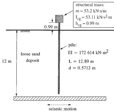
Fig. 5. The finite element modelling of the single pile.
