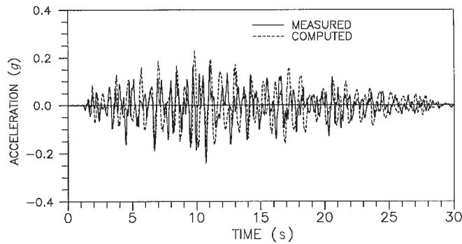
pile cap is  $0.23g$ , which agrees very well with the measured peak acceleration of  $0.24g$ .
