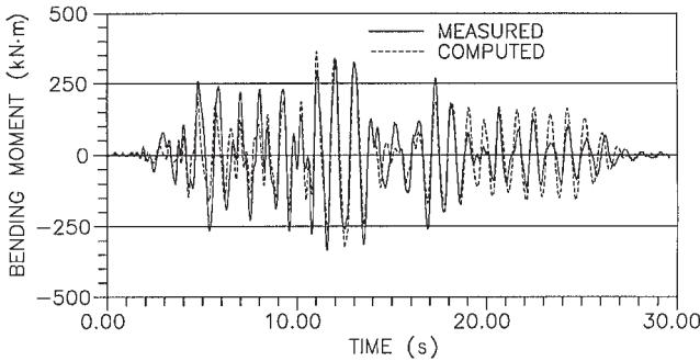
**Fig. 9.** Comparison between measured and computed bending moments at peak pile deflection for the single pile.
