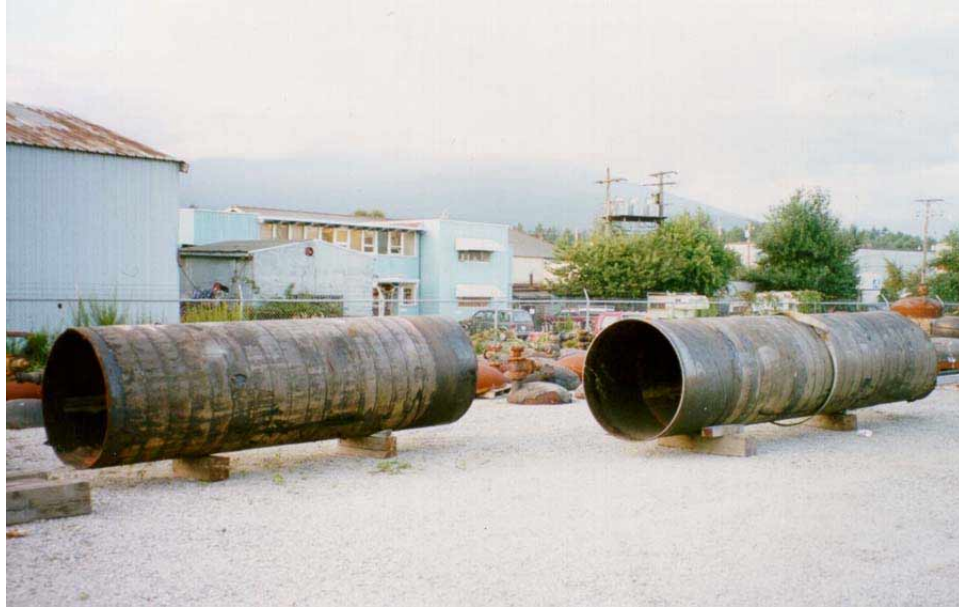
Figure 6 Port Mann Crossing Salvaged Piping used for Bell and Spigot Joint Fabrication
